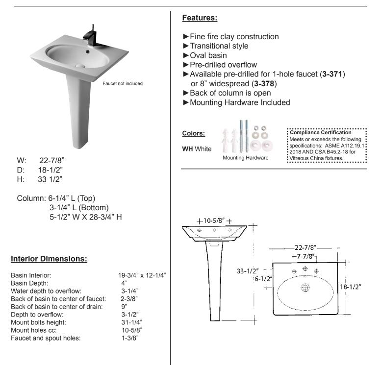
Dimensions of fixture are nominal and may vary within the range of tolerances established by ASME Standard A112.19.2-18. Dimensions and specifications subject to change without notice.
